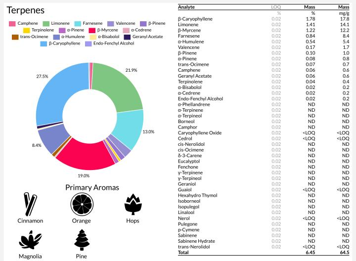
Date Tested: 12/17/2020; Analysis performed on Agilent 7890A GCFID
